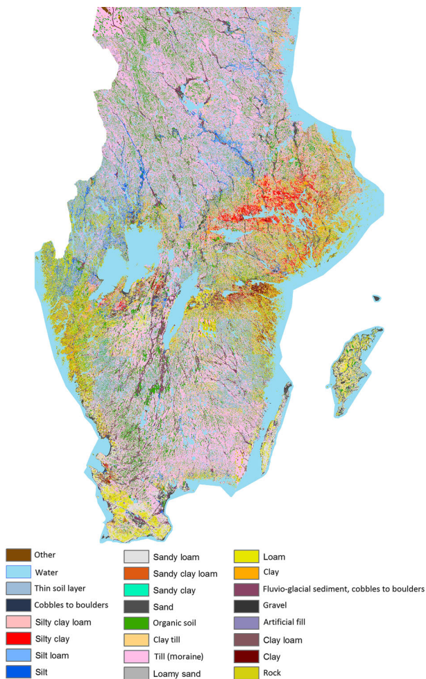
Fig. 4 Soil texture and other materials distribution map used for erosion modelling. The map is based on the Digital Arable Soil Map of Sweden (Söderström and Piikki 2016) for agricultural land and soil maps from the Geological Survey of Sweden for non-agricultural areas
